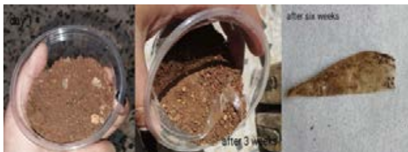
Fig2. Biodegradability test showed degradation after 3 & 6 weeks with loss of volume.
