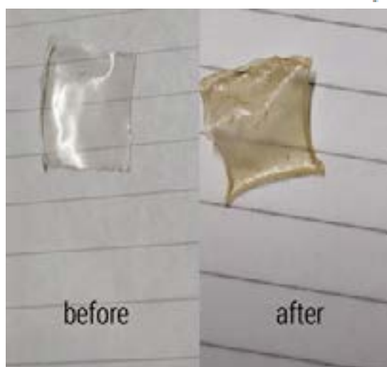
Fig1. A comparative image of a bioplastic sample before and after heating in an oven with visually observed changes.
